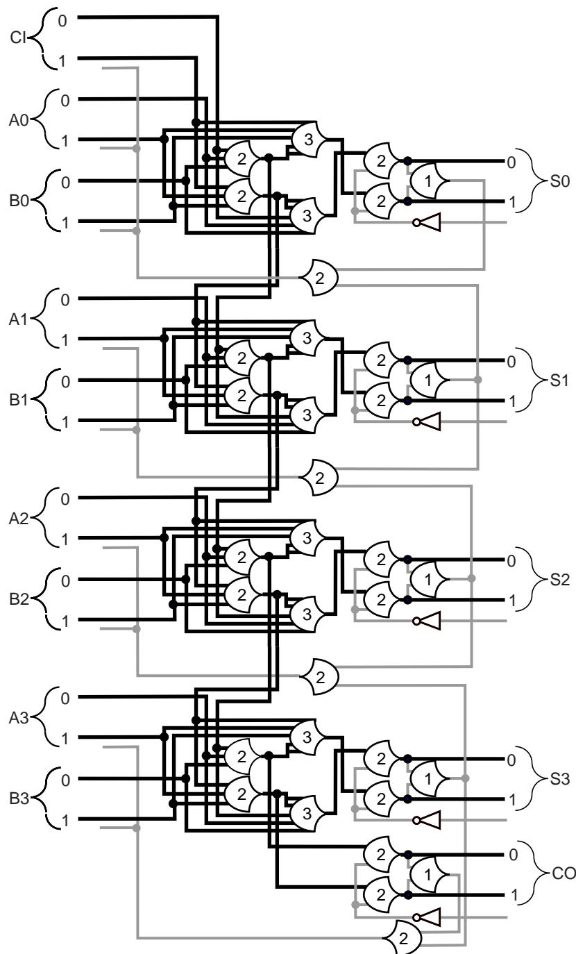
The carry is pipelined indirectly by sharing a completeness behavior
