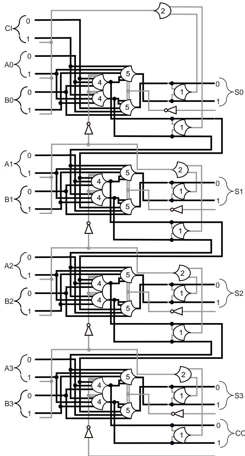
The enable ranks of the links are integrated with the combinational logic
